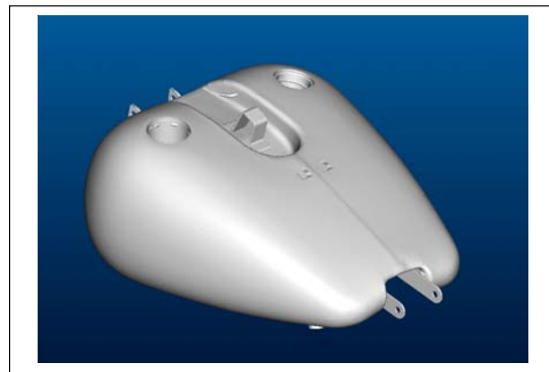
Figure 5. Great products are a perfect wedding of customer interests. There’s something visually old, to capture favorable associations. There’s something visually new, to create excitement. Harley-Davidson is an icon in its industry in part because it understands this balance. This “retro” tank design for a new Harley is based on sampling a customer favorite from the past. Scanned data from the old tank was used as a starting point for the new design. Image courtesy of Advanced Design Concepts (Pewaukee, Wisc.) and Harley-Davidson (Milwaukee).
