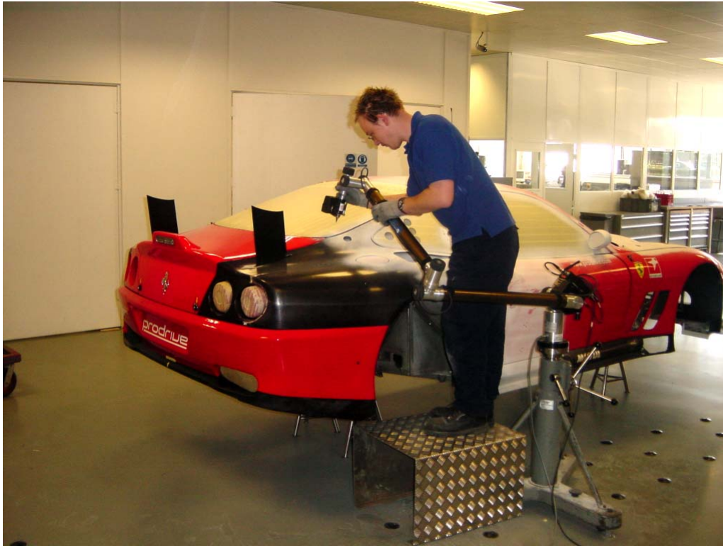
Figure 11. The ProDrive Ferrari team uses DSSP and CFD (computational fluid dynamics) to optimize aerodynamics. Image courtesy of 3D Scanners (London).
